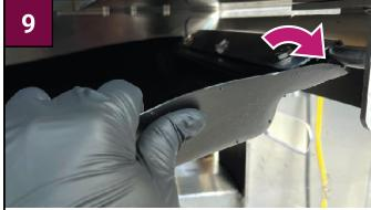
Hook the upper end onto the support rail.
