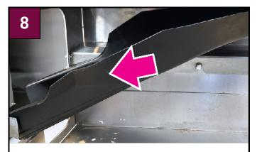
Install the Dispenser Chute by passing the bottom end through the hole on the side barrier.
