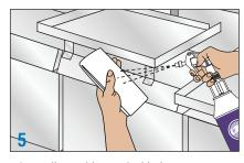
Spray disposable towel with degreaser solution and wipe fryer shelves, fryer and basket markers and any soiled parts of machine and frame including autobasket rack drawers, handles, panel area, elevator carriage, and fryer localization.
