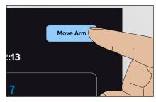
Close barriers, release E-stop, and press "MOVE ARM" on display. Arm will move to other side of the machine. Open barrier and repeat step 7 on previously blocked plexiglass.
