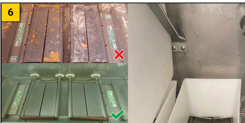
Be certain that all food debris has been removed before replacing the Accumulator.
